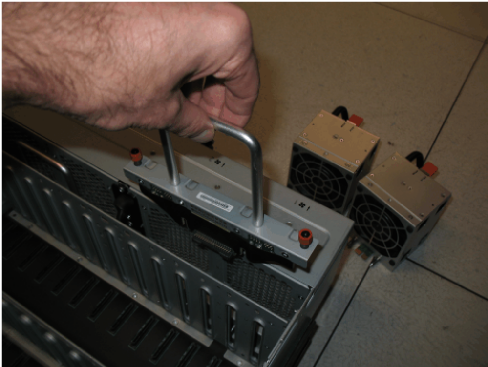
Figure 93. Insert the new FIB in the chassis
